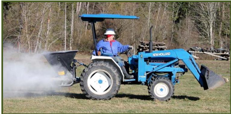
*Lime being spread with the KCD Broadcast Spreader*
