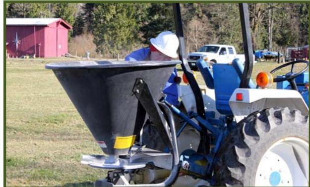
*The PTO-driven cone broadcast spreader*
