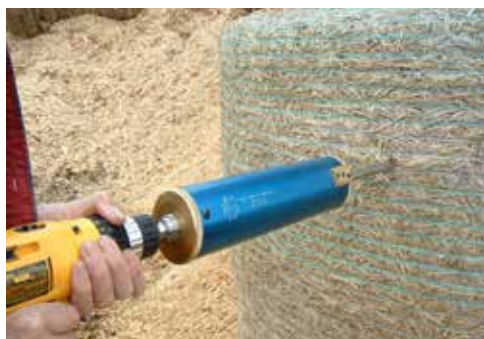
Taking a core sample with drill (14 volt or greater is recommended)
